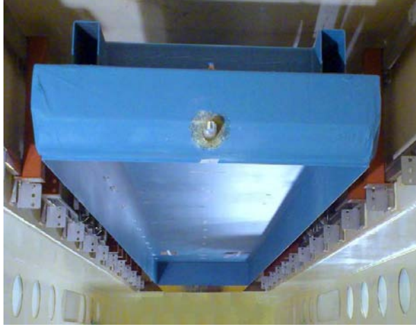
Figure 5: Cavity box installed in the upper chamber of test section.
