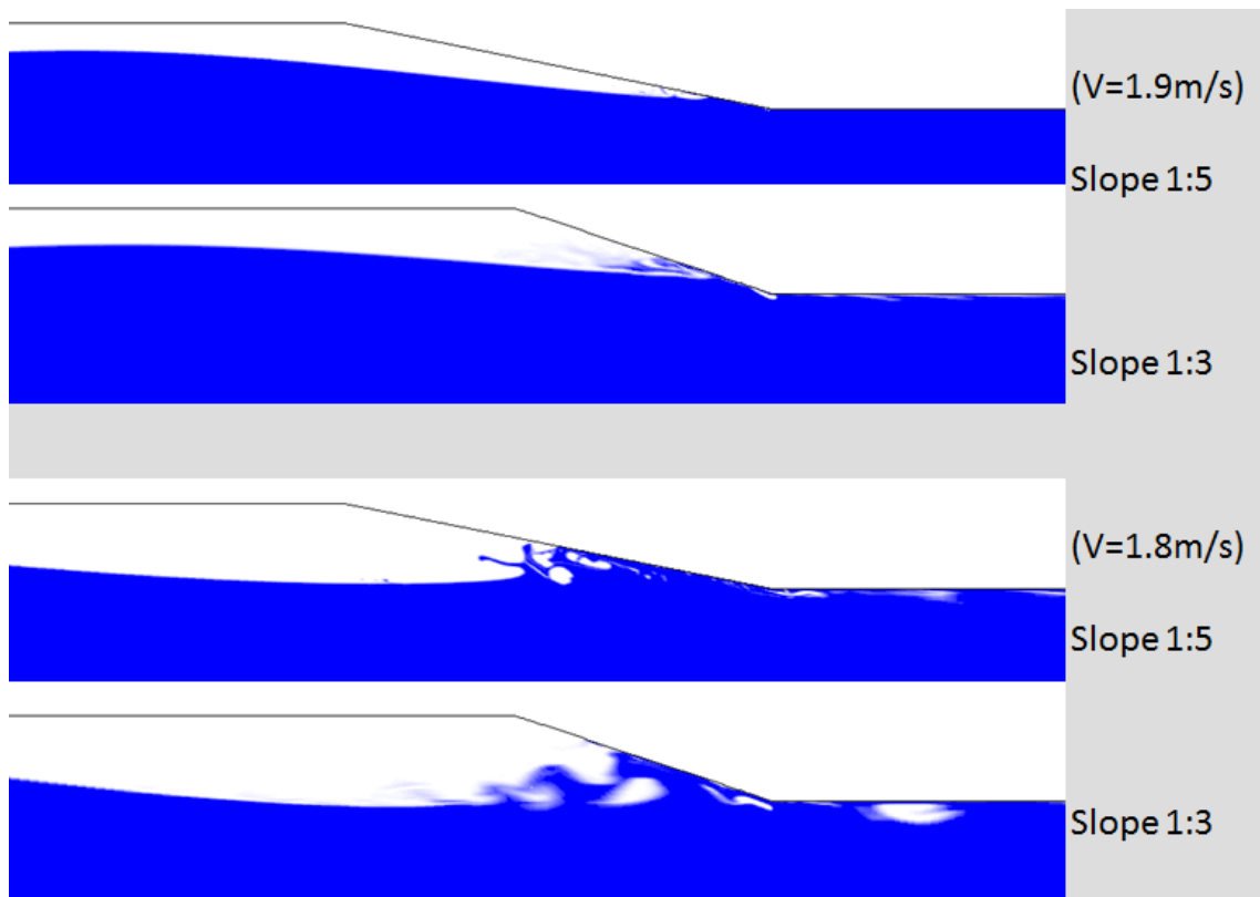
Figure 9 - 2D Simulation; beach re-attachment angle in different velocity and beach slope.
