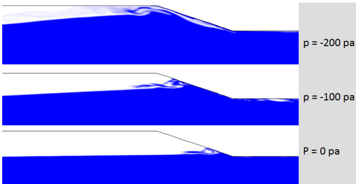
Figure 6 - 2D Simulation, beach re-attachment angle in different pressure.
