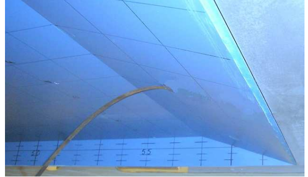
Figure 6: Beach plate and the side wall lines for measuring water surface height.
