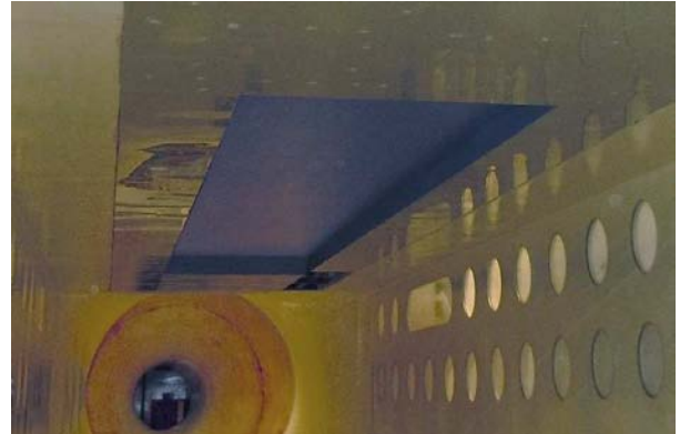
Figure 8: Side windows of the test section. The second camera was recording movies of the beach plate through these windows.
