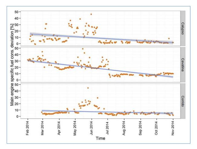
The comparisons show an approx. variation of in between 0-25% for the ME SFOC (when removing impossible erroneous readings) at different ME load. The comparisons do also show that the wrong readings, prior final commissioning of the installed AE MFM's, has been substantially reduced and can now be considered as being close to manufacturers claimed SFOC (see orange/red measurements in above diagrams).
