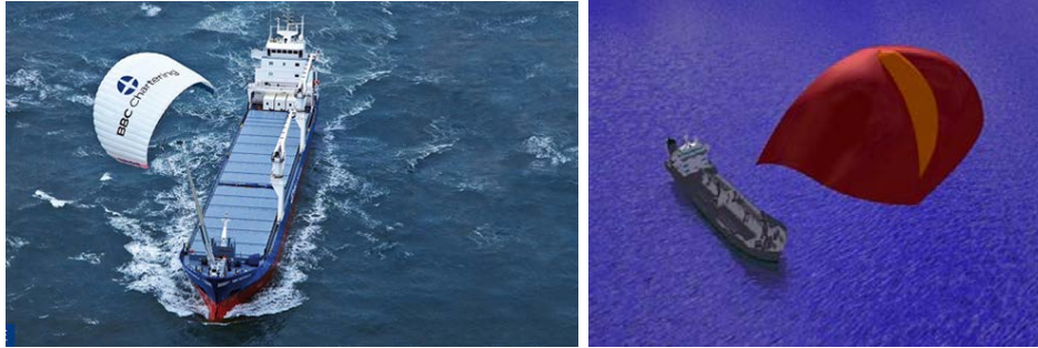
Figure 5: (Left) A SkySails towing kite implemented in oceangoing commercial vessel, and (right) another kite propulsion concept developed by Kiteship.
