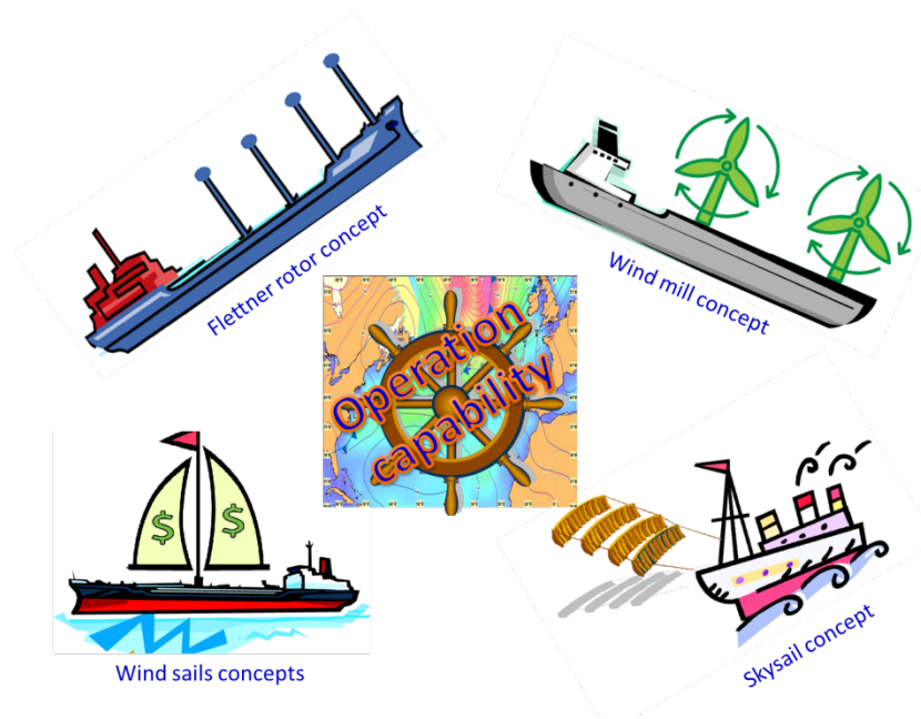
Figure 3: Different green shipping concepts using wind power as auxiliary propulsion.
