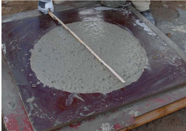
Figure 13: Slump flow of tested SCC, measuring approximately 700 mm.
