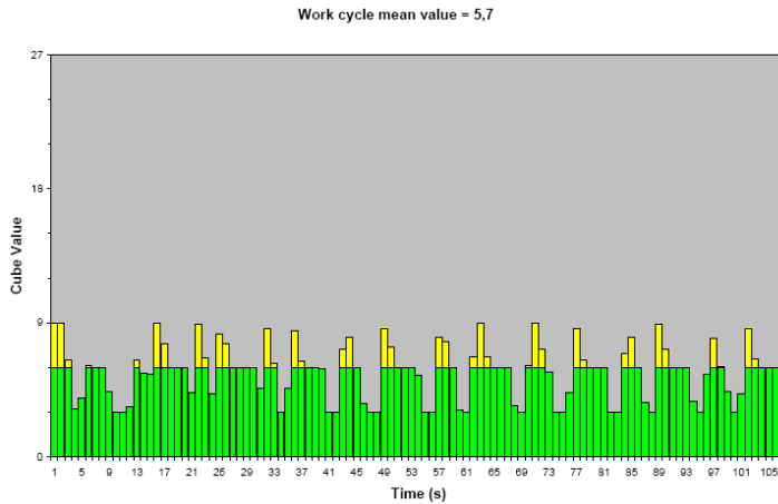
Figure 24. ErgoSAM analysis of concrete worker's short work cycle during SCC casting.
