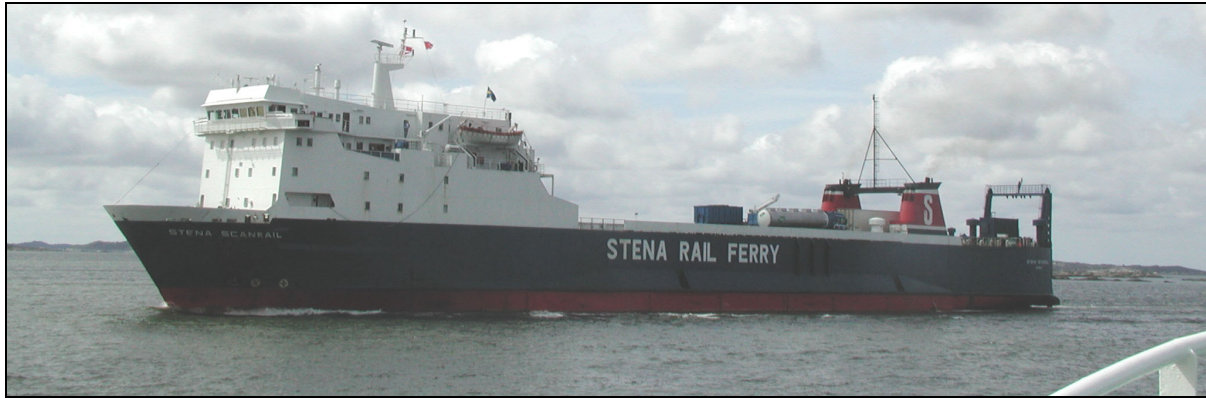
Figure 9a. The freighter Stena Scanrail (photo taken on June 15 th ). This freighter is running on fuel with 2% sulfur content, according to the shipping company. The gross tonnage is 7504 tons.
