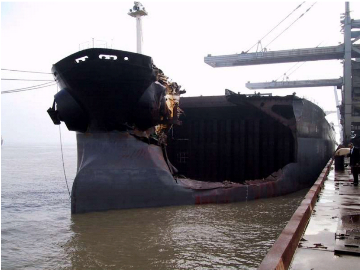
Figure 2 A VLCC in ballast after a collision with a fully loaded cape size bulkship. The collision angle was about 45 degrees
