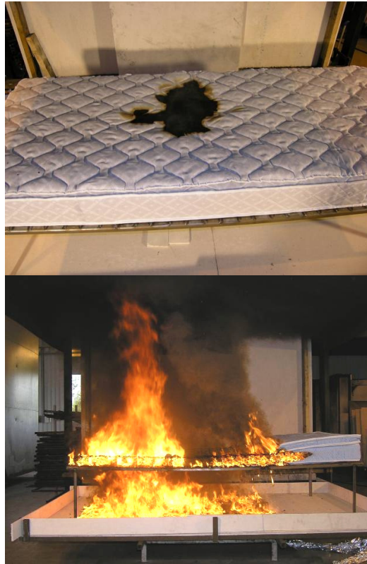
Figure 5.1 The difference between the fire performance for two mattress types is illustrated in the above photographs. The mattress on the upper picture has high resistance to ignition and exhibits other good fire performance properties, while the mattress on the lower picture clearly has much worse fire performance properties.
