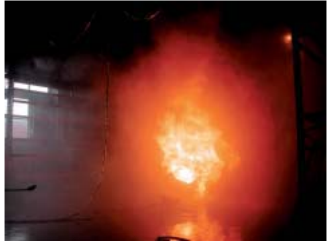
Figure 2: The entire DESSO ROPAX is protected by a high-pressure water mist system. A fire in a machinery space is shown above immediately after engagement of the system, and before the fire has been fully controlled.
