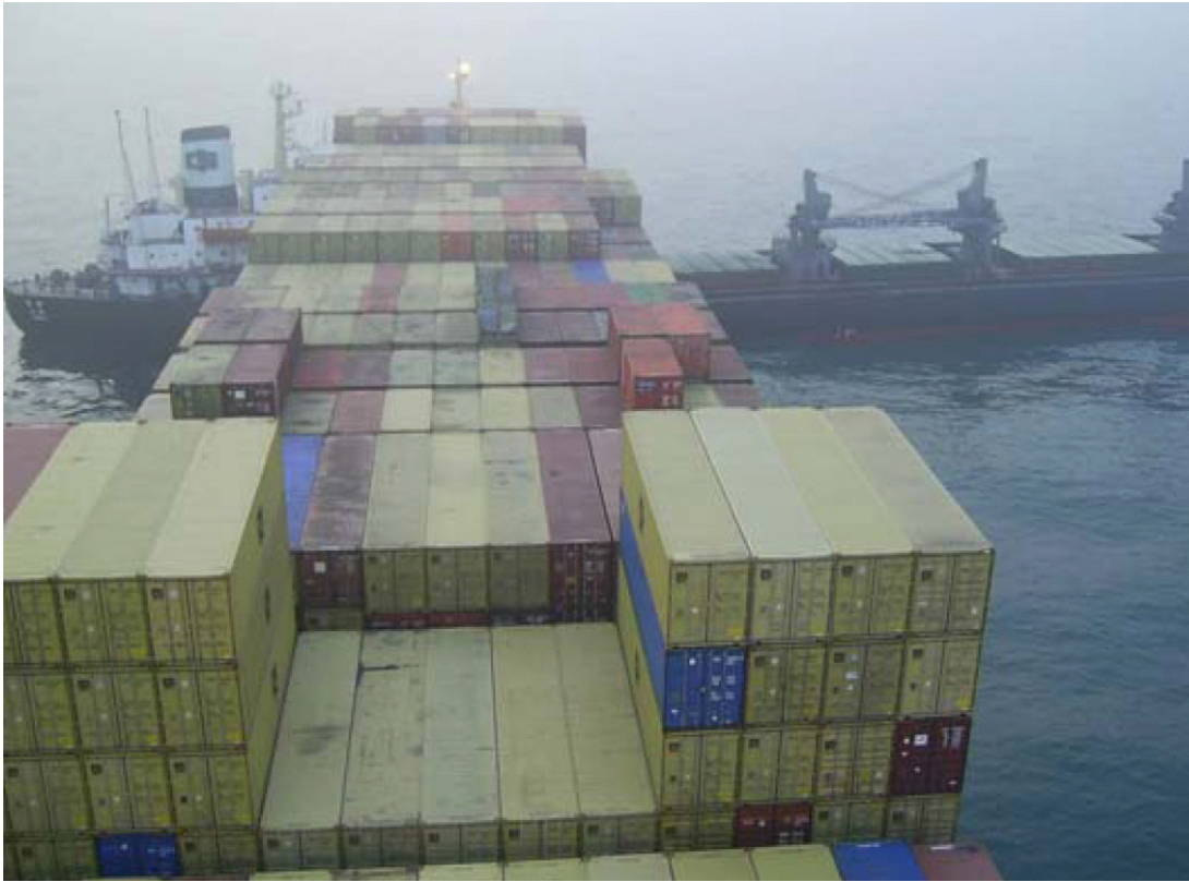
Figure 1 A Panamax container ship in collision with a handymax/general cargo ship.
