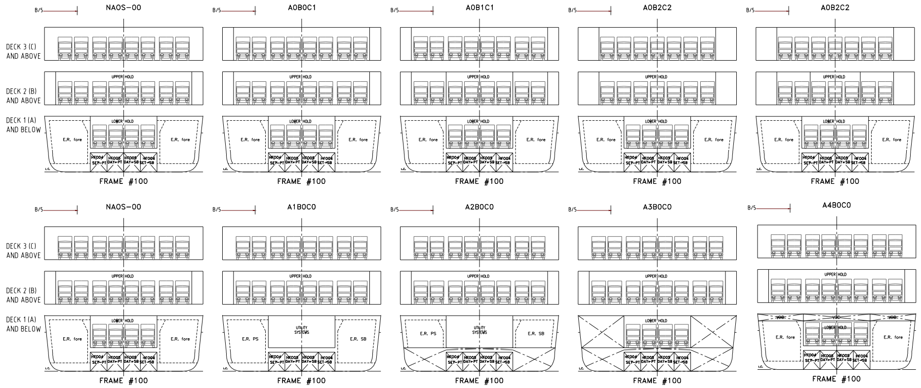
Figure 16 First Concept Generation - Alternative Watertight Integrity Arrangements
