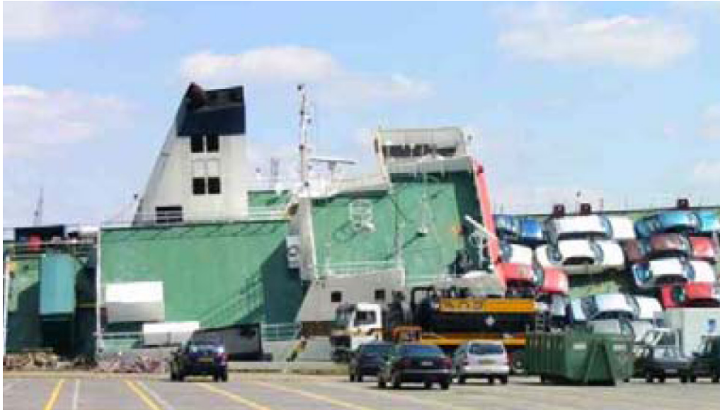
Figure 7 Fire extinguished but the ship heeled over due to free water surface from fire fighting
