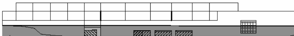
Figure 11 The transverse bulkheads is located at the thick lines through the lower casing.
