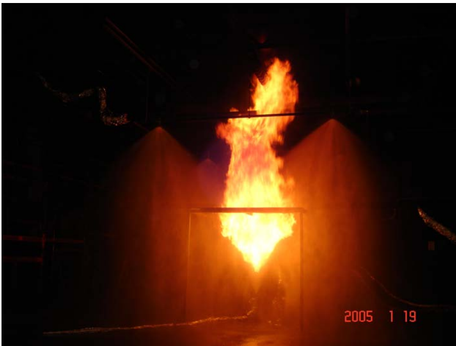
Photo 4 The 3,5 MW diesel spray fire at the 5,0 mm/min water discharge density.
