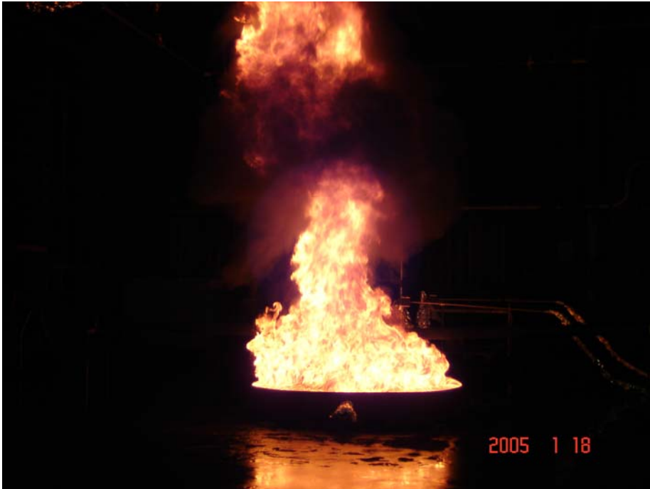
Photo 1 Free-burn of the 3,5 MW diesel pool fire.
