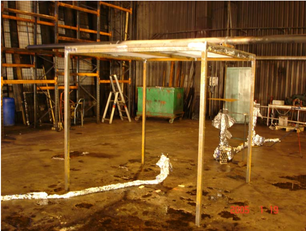
Figure 6 The oil spray nozzle was positioned 500 mm above floor and directed vertically upward towards a steel grating.
