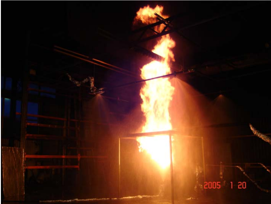
Photo 5 The 3,5 MW diesel spray fire at the 7,5 mm/min water discharge density.
