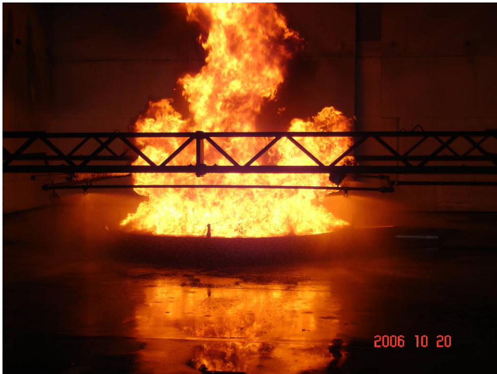
Photo 14 Test 10: The water discharge density of 7,5 mm/min provided 'limited fire control'.
