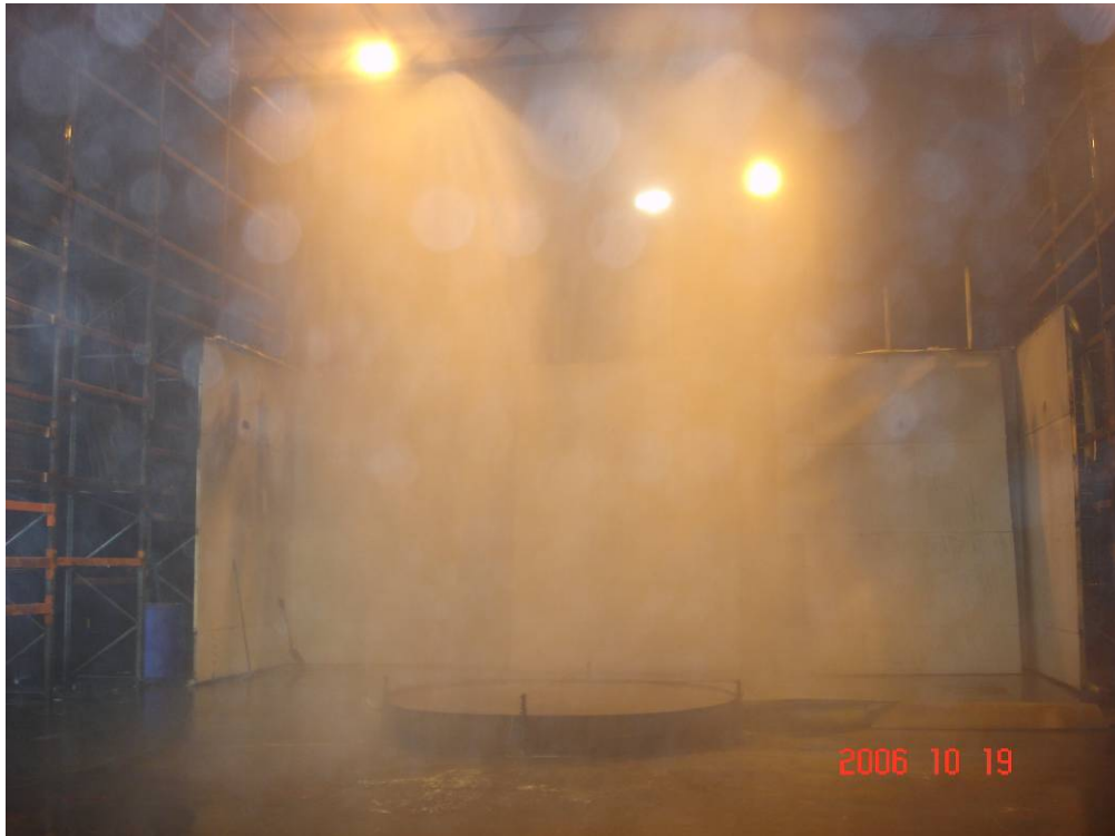
Photo 13 Test 7: Fire extinguishment at 02:10 [min:sec].
