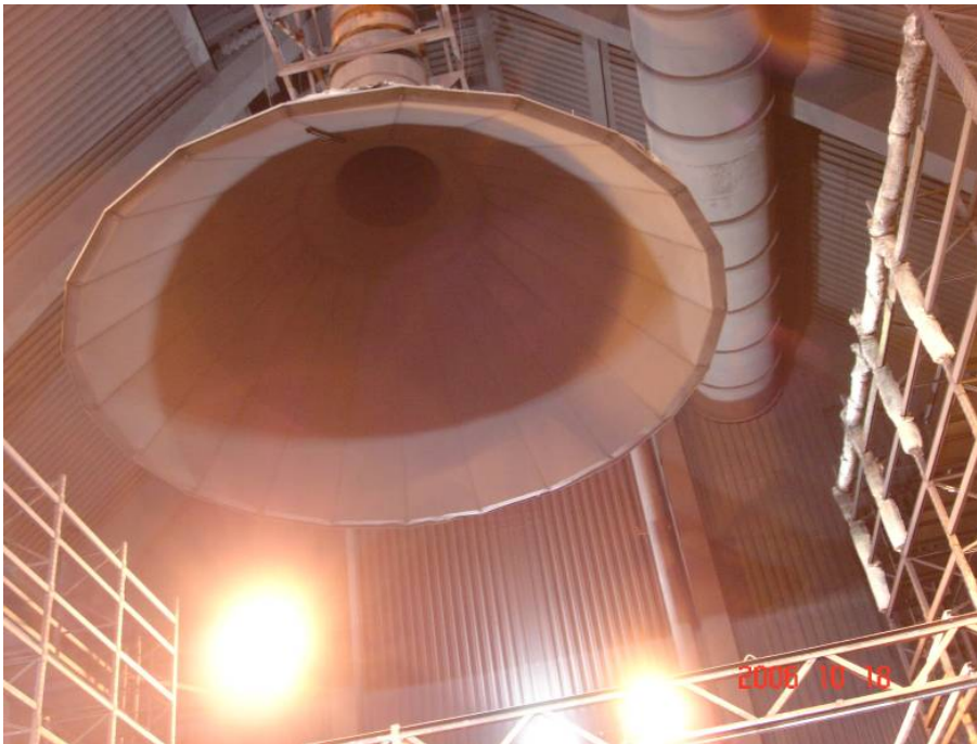
Figure 1 The Industry Calorimeter was used to measure the convective Heat Release Rates from the fires.
