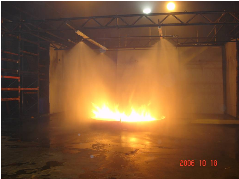
Photo 5 Test 1: The fire was suppressed almost immediately.
