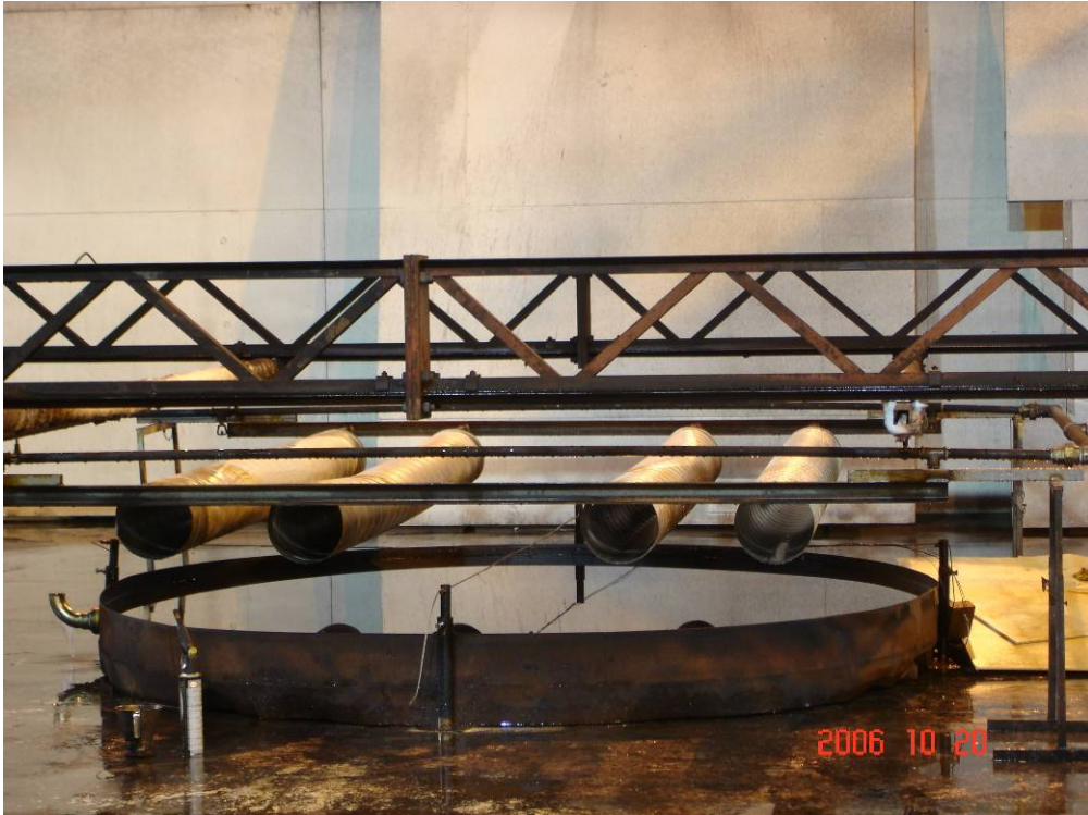
Photo 17 The four Ø=250 mm steel pipes that was used to obstruct the pool fire surface in Tests 12 and 13, respectively.
