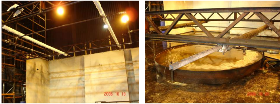
Figure 3 The system pipe-work when positioned at the 'high' elevation (left hand photo) and at the 'low' elevation above the pool fire tray.
