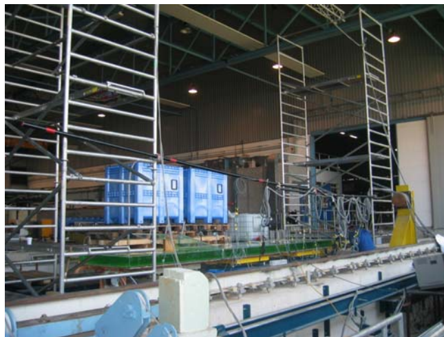
Fig. 4. The MV Estonia test set-up on the platform of the SMB basin of MARIN.
