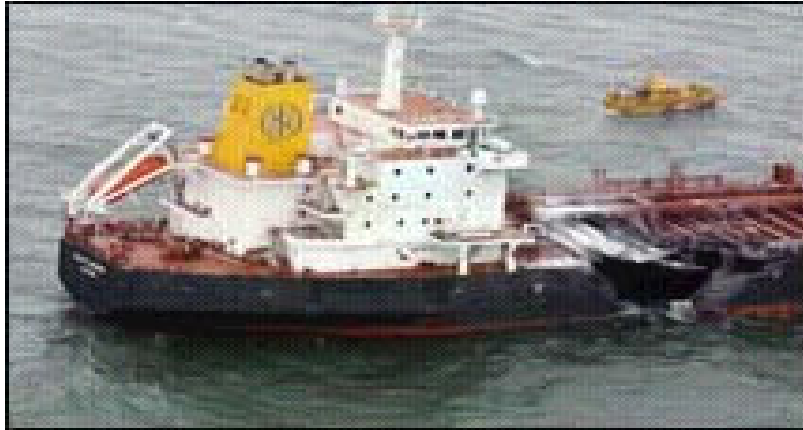
Photo 7.2: The tanker's hull holed after collision with the bulk carrier ship. Source: AP
