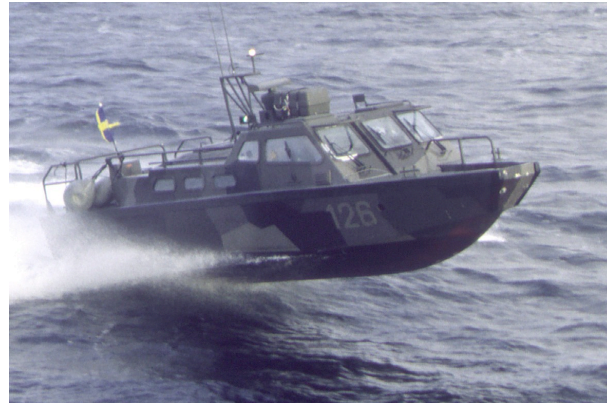
Figure 3: High-speed craft Storebro 90E, used for instance by the Swedish navy and operates in speed regimes up to and above 40 knots (photo: Anders Rosén).
