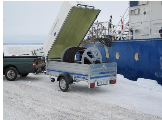
Picture 3. The sludge hose cart at the dock.
