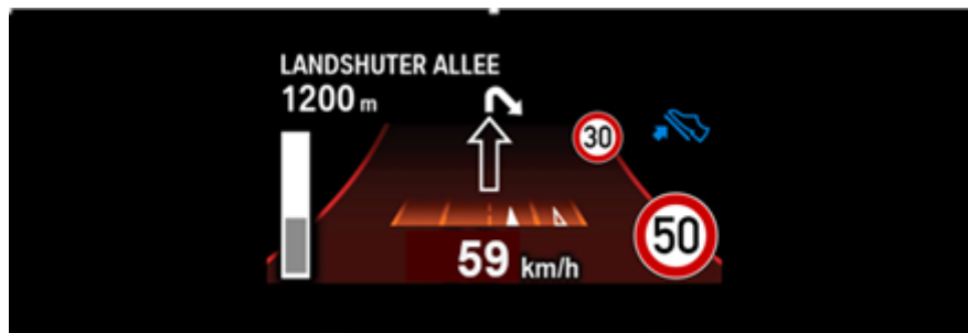
Figure 18: Coasting advice provided in the HuD (here for a lower speed limit).
