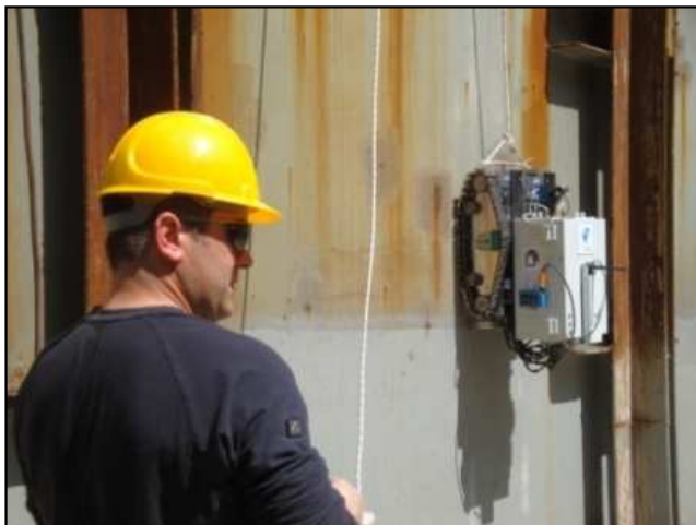
Fig. 11: The CNR magnetic crawler
