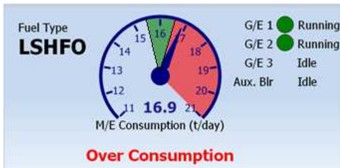
Fig. 4: M/E fuel oil over-consumption and status of generators
