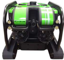
Fig. 7: vLBC with vortex suction system
