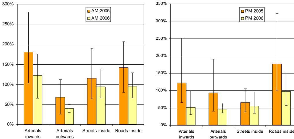
**Figure 4. Relative increase of travel times for various categories of links. 0 percent corresponds to free-flow travel time. The coloured bars show average travel times while the "error bars" indicate the worst decile and the best decile of the travel time distribution. Measurements were taken from all weekdays for six weeks in April-May. "AM peak" refers to 7.30-9.00, "PM peak" refers to 16.00-18.00.**
