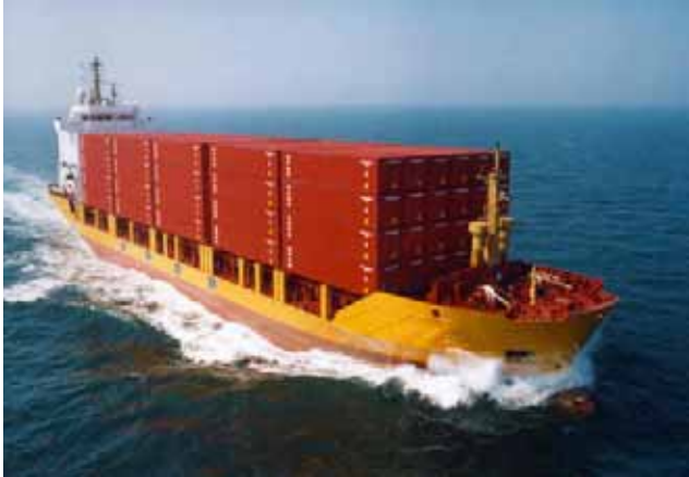
Figure 26: Typical container ship having a tower as accommodation and low freeboard
