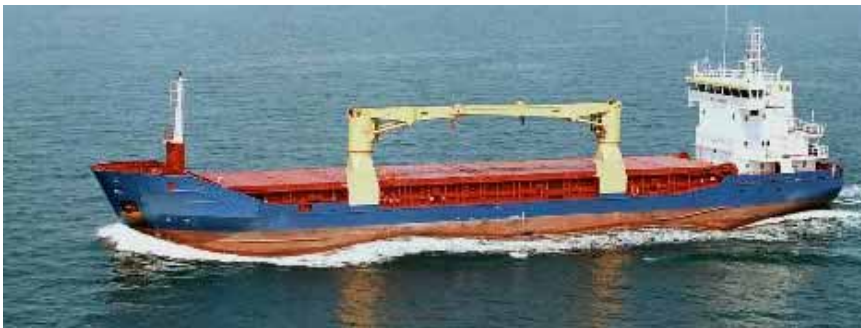
Figure 27: A general cargo vessel prioritise the volume in the hold and is often geared
